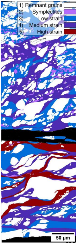
Figure 11: Schematic overlay of strain localization in Type III-cg experiment 675NN. SEM-BSE image of large clast from the bottom surrounded by high strain grains is displayed in Fig. 3.
