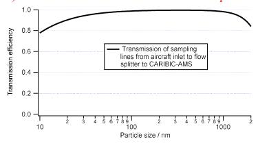
3) Transmission of the plumbing inside the CARIBIC-AMS rack (1/8"lines, flow 0.3 l min<sup>-1</sup>), measured in the laboratory and calculated:
