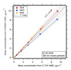
We still think that the figure is useful because it shows the reproducibility of two different AMS instruments. To our opinion, a comparison with well defined (350 nm) laboratory generated aerosol particles appears favourable over a comparison with unknown ambient aerosol.
