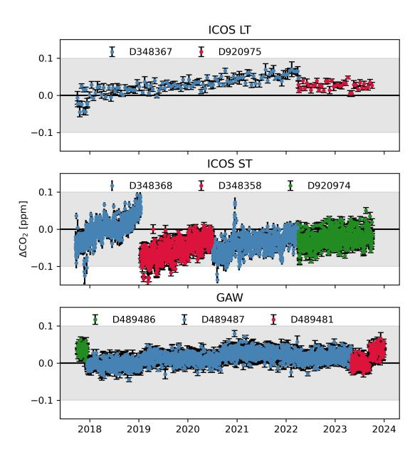
Figure 7. CO2 target measurements of ICOS LT, ICOS ST and GAW target cylinders over the whole comparison period. Different cylinders used are marked with distinct colors. The data are given as means of each sequence with the associated standard deviation.
