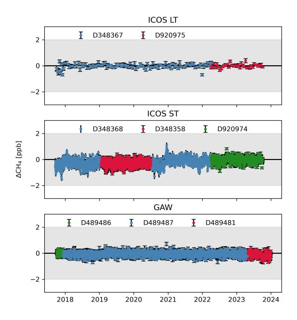
Figure 13. CH4 target measurements of ICOS LT, ICOS ST and GAW target cylinders over the whole comparison period. Different cylinders used are marked with distinct colors. The data are given as means of each sequence with the associated standard deviation
