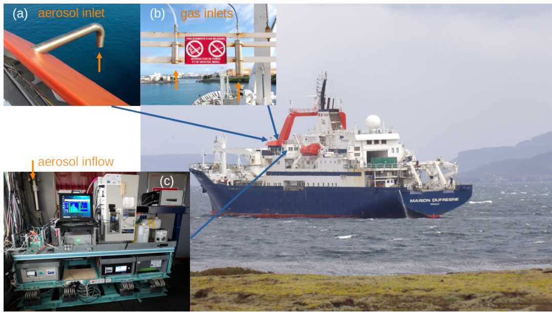
Figure 3. Picture of the Marion Dufresne in the Port-aux-Français Bay (February 2024). (a) The aerosol and (b) gas inlets are located above the wheelhouse. (c) The acquisition and monitoring system is located in the meteorological room, next to the wheelhouse and mounted above a shock-absorbing table. Aerosol monitoring systems are on the top shelf, right of the acquisition computer. Gas analyzers are on the bottom shelf. Photography credits: Meredith Dournaux.
