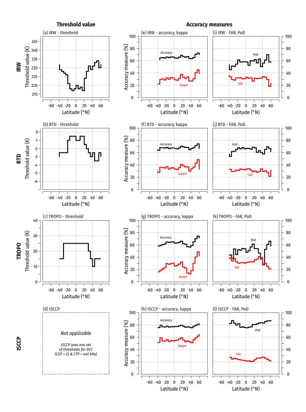
**Figure 2**. The optimal threshold for each method as a function of latitude (a–c), together with corresponding latitude-resolved measures of accuracy. Kappa ( $\kappa$ ) values were multiplied by 100 to match the 0–100% range.
