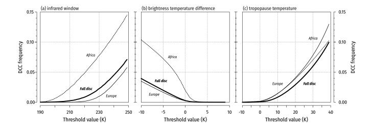
**Figure 4**. Mean seasonal (June-July-August 2005) DCC frequency as a function of the threshold applied to the DCC detection methods evaluated in this study. The frequencies are given in the range <0,1>, where '0.0' indicates a DCC-free sky and '1.0' indicates DCC occurring consistently across the sky.
