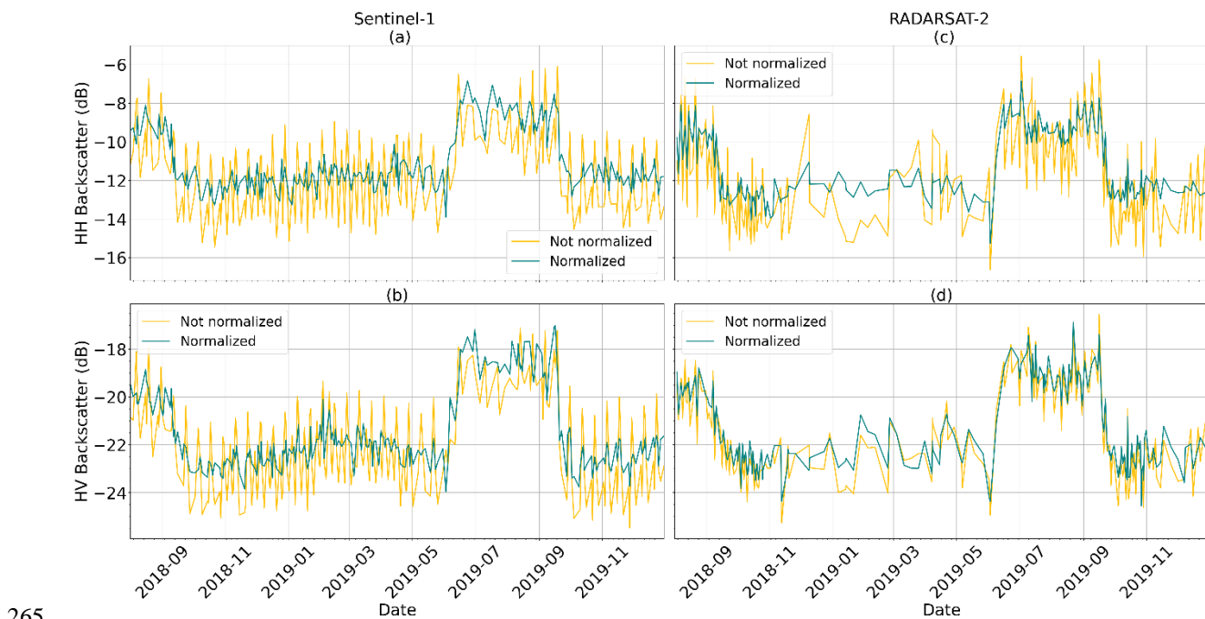
Figure 4: Examples of the backscatter time series for one pixel of Sentinel-1 and RADARSAT-2 data for the study period after basic preprocessing (yellow) and incidence angle normalization (green).
