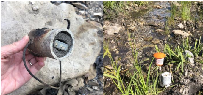
1551 Figure 44-12. Monitoring inundation regimes is increasingly possible via in situ sensors. 1552 Stream Temperature, Intermittency, and Conductivity Sensors (STICs) (Chapin et al. 1553 2014 )(Chapin et al. 2014), one of the types of increasingly available sensors to measure water 1554 presence/absence in an inexpensive and easily deployable manner. These sensors can be used 1555 across all types of VIEs. Credit: Amy Burgin.
