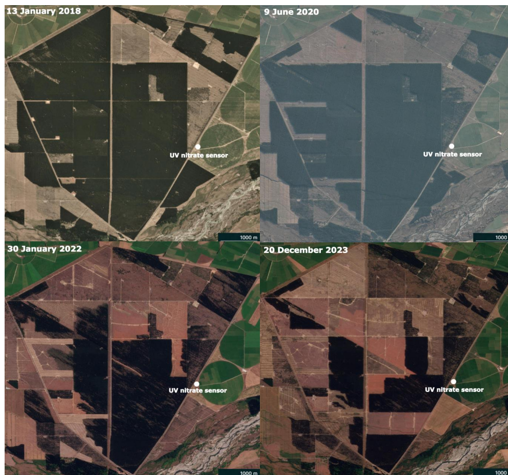
Figure 6: Land use cover changes from daily PlanetScope imagery (3 m resolution) showing the reduction in forestry cover from 2018 to 2023 (Planet, 2024)
