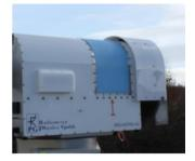
The radome is made of blue foam with an hydrophobic coating. Ageing takes the coating off. We added this information in the manuscript.
