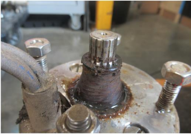
20 Figure SI 1: State of the submersible pump after running for five months during the high flow, winter period at the Naizin catchment. Deposition of primarily organic material within the hydraulic parts of the pump and strong wear of the mechanics can be seen.
