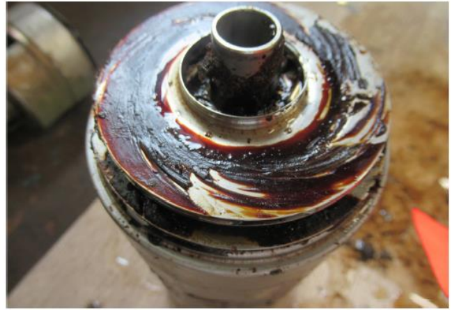
20 Figure SI 1: State of the submersible pump after running for five months during the high flow, winter period at the Naizin catchment. Deposition of primarily organic material within the hydraulic parts of the pump and strong wear of the mechanics can be seen.
