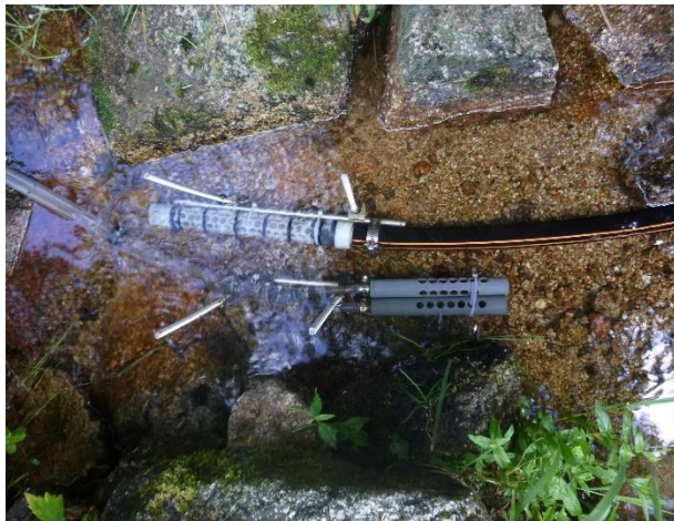
560 Figure 3: Pictures of the strainers and baffles in the station of Naizin (top) and Strengbach (bottom) to prevent clogging of the pumps.
