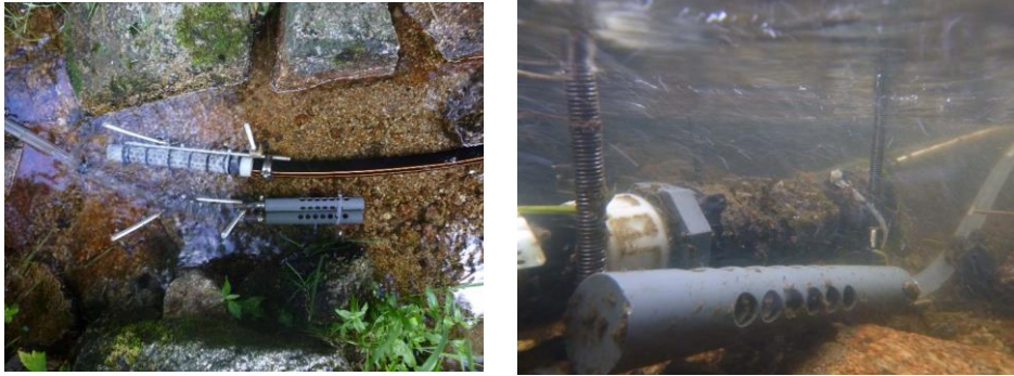
Figure 3: Pictures of the strainers and baffles in the station of Naizin (top) and Strengbach (bottom) to prevent clogging of the pumps.
