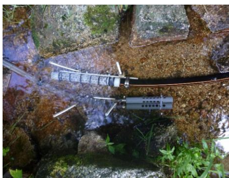
Figure 3: Pictures of the strainers and baffles in the station of Naizin (top) and Strengbach (bottom) to prevent clogging of the pumps.
