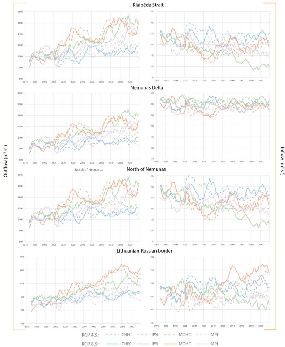
268 269 Figure 3. 10-year moving average graphs of outflowing (left column) and inflowing (right column) water fluxes (in m^3 s^{-1} ) 270 across four cross-sections within the Curonian Lagoon. Note the adjusted y -axis ranges for fluxes passing through the 271 Lithuanian-Russian border.
