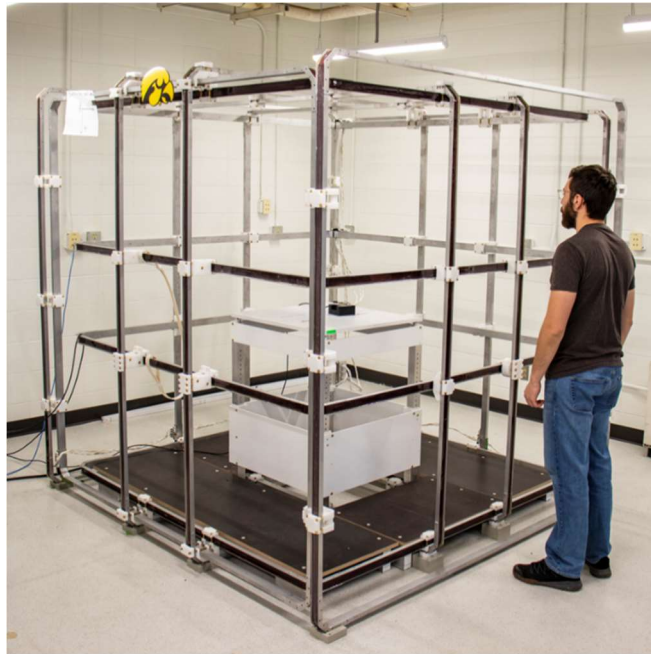
Figure 2: Merritt coil system used to simulate various geophysical signals.
