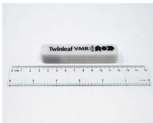
Figure 1: Twinleaf VMR magnetometer used in the generation of this dataset.
