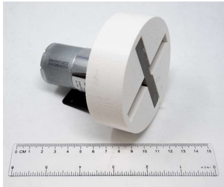
Figure 3: Low-frequency motor and attached plate with inset cast iron strips, designed to simulate spacecraft reaction wheels.
