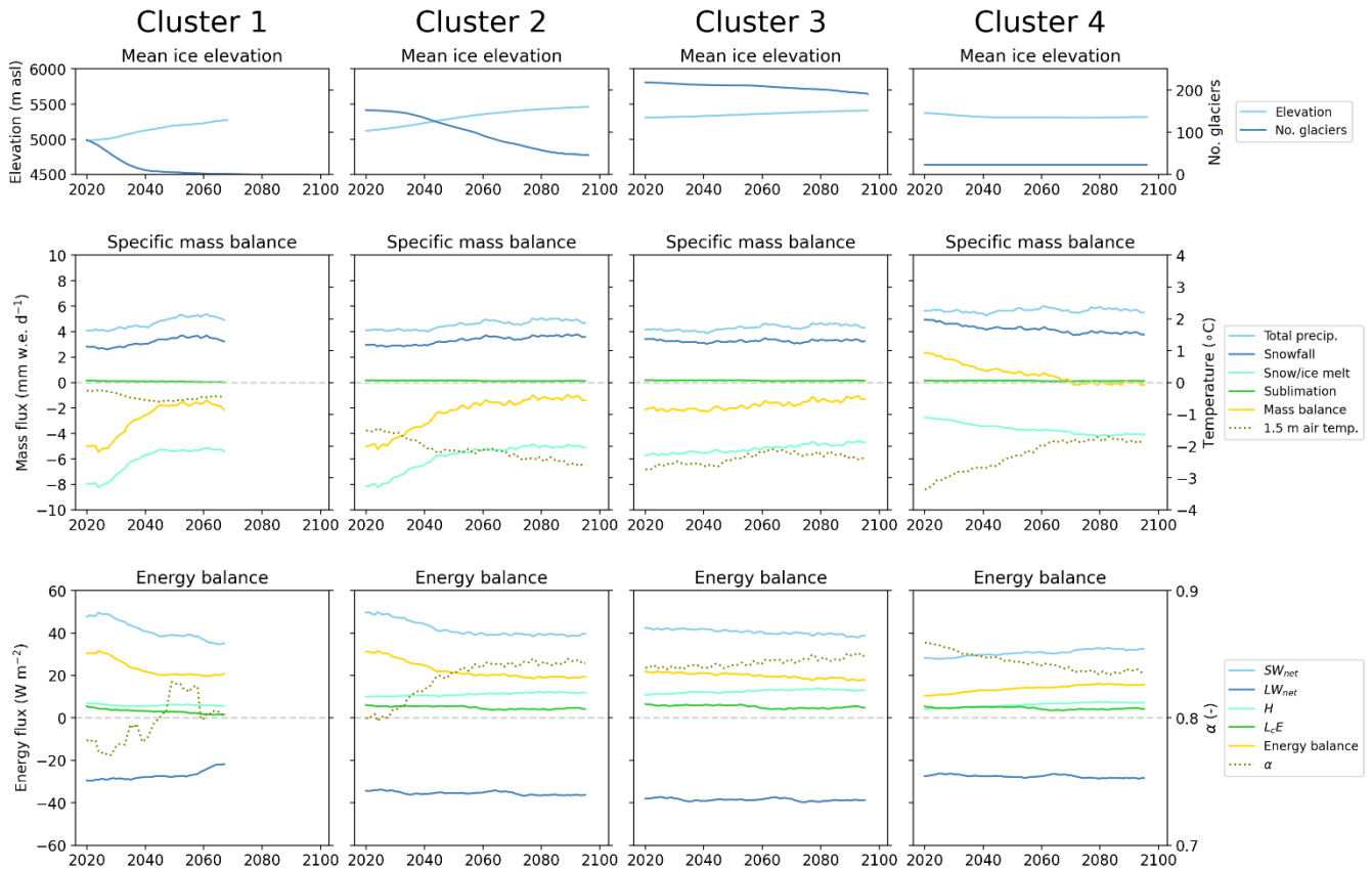
E 1: Simulated mean glacier-wide state-variables from JULES-OGGM between 2020 and 2100 for each cluster (columns) and based on the BNU-ESM simulation under RCP4.5. The variables include ice elevation (top row), specific mass balance (middle row) and energy balance (bottom row). All variables are calculated over a 10-year moving average window and are taken as the mean across all glaciers within a cluster, weighted by the glacier area.
