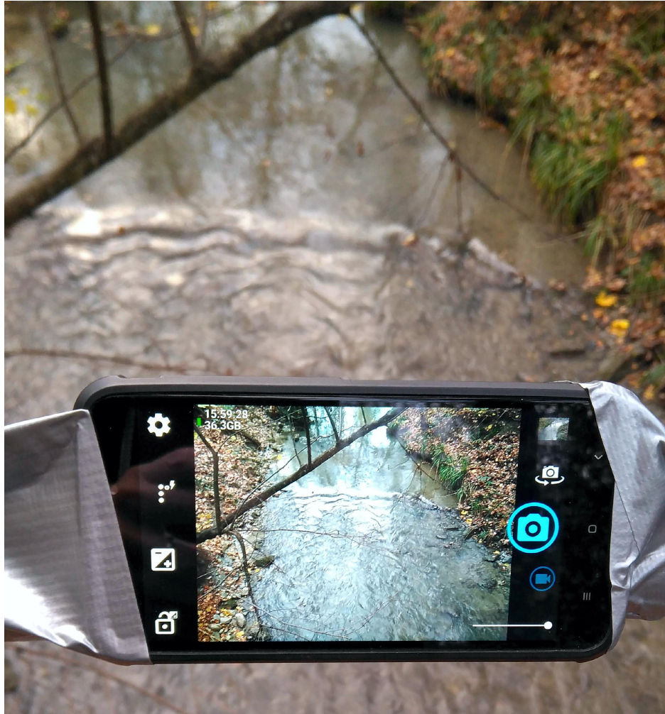
Figure B1. Example image data acquisition (dataset 5). A mobile phone camera was securely mounted using duct tape, providing a stable view of the river's surface from a bridge.
