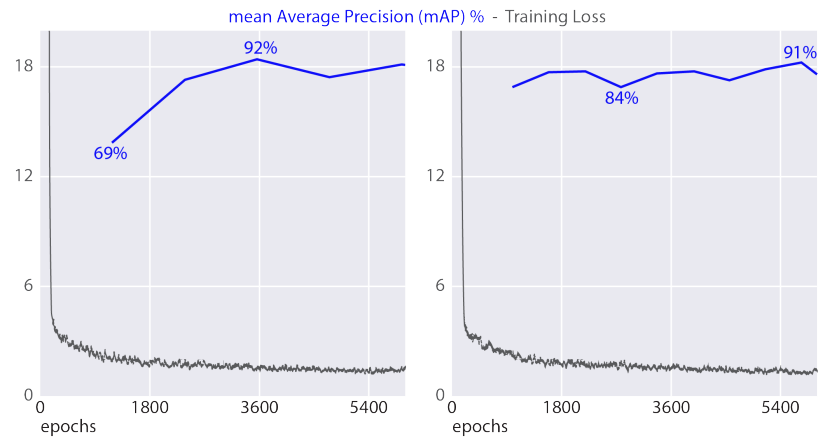
Figure 6. Training performance of dataset 13 (see Table 1) when using 2,000 images (left) and 500 images (right) per dataset (respectively 38,000 and 9,500 training images used). Blue: mean Average Precision, Grey: Complete Intersection-Over-Union Training Loss (Zheng et al., 2020)
