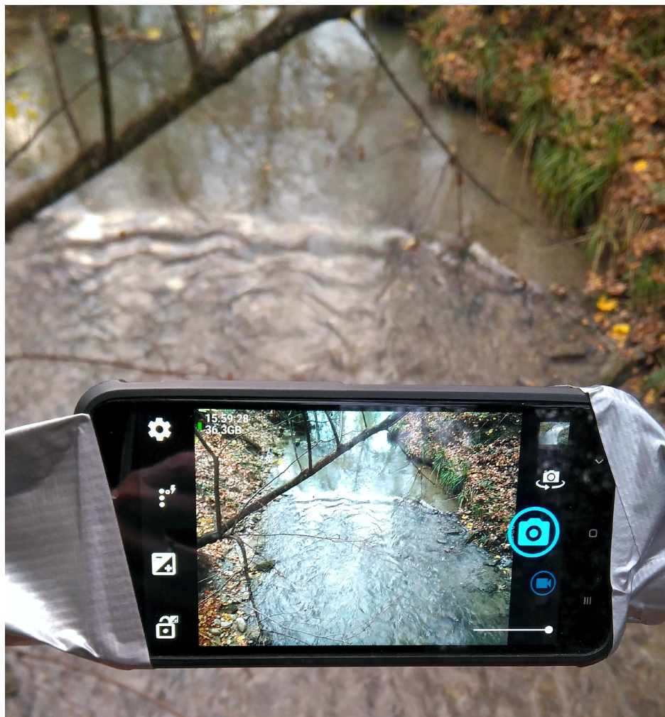
Figure B1. Example image data acquisition (dataset 5). A mobile phone camera was securely mounted using duct tape, providing a stable view of the river's surface from a bridge.
