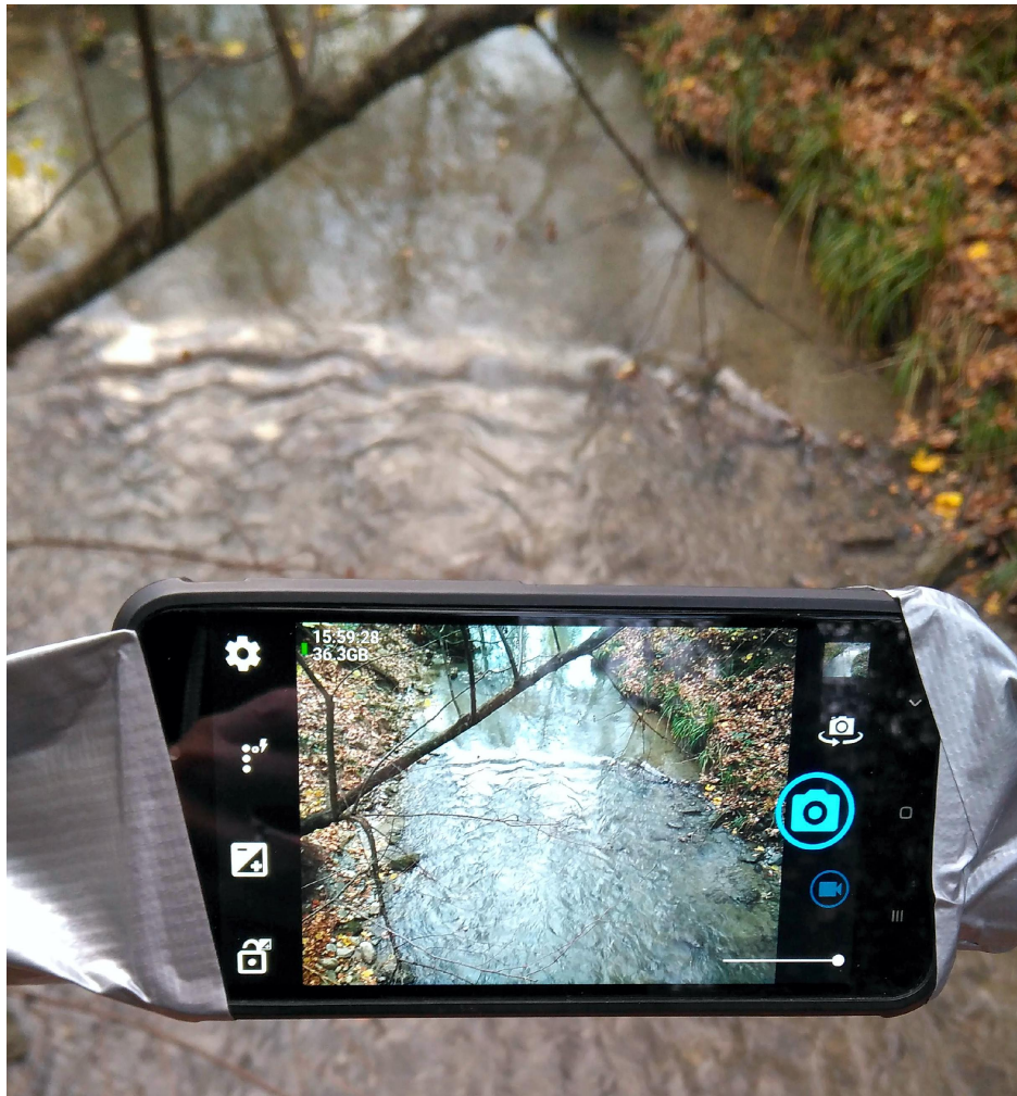
Figure 03. Example image data acquisition (dataset 5). A mobile phone camera was securely mounted using duct tape, providing a stable view of the river’s surface from a bridge.
