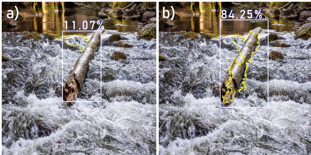
Figure 8. Wood detections according to the models trained with the a) Baseline scenario and b) Scenario 9. We indicate the heaviest weighting pixels in yellow according to the neural networks.
