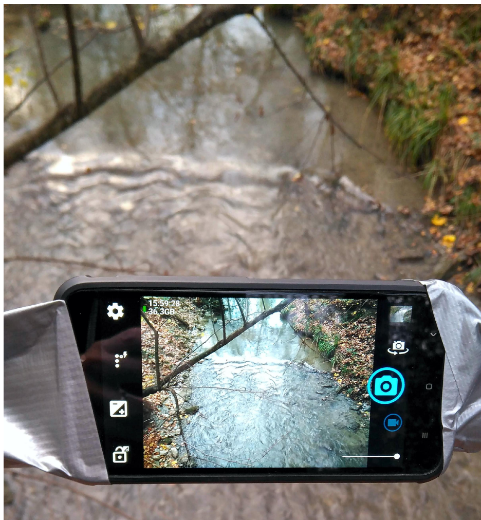
Figure 13. Example image data acquisition (dataset 5). A mobile phone camera was securely mounted using duct tape, providing a stable view of the river’s surface from a bridge.
