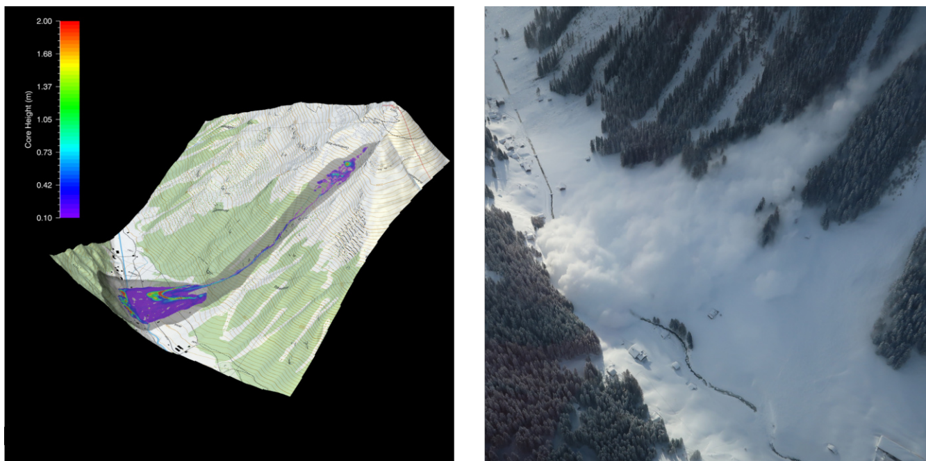
Figure 15. Simulation of the powder cloud accompanying the Ruechi avalanche (left) simulation and (right) photo of the cloud taken from the helicopter (map source: Federal Office of Topography).
