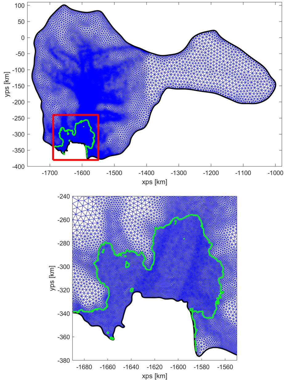
**Figure B1.** Initial mesh for the Pine Island Glacier model domain. Catchment area is encompassed by the thick black line and the linear triangular mesh elements are shown in blue. The red square in the top plot outlines Pine Island Ice Shelf which is enlarged in the lower plot, and both show the grounding line in green.
