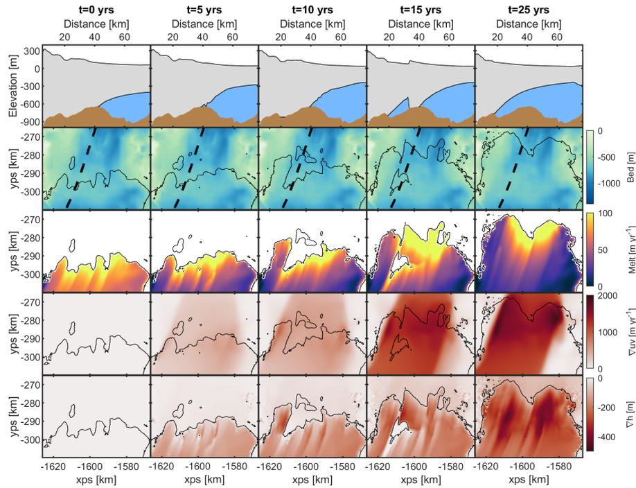
**Figure 4.** Evolution of flowline profiles (**top row**), grounding-line position over bed elevation (**second row**), basal melt rate (**third row**), change in ice speed (**fourth row**) and change in ice thickness (**bottom row**) during the WARM25 experiment. The columns from left to right show results after:  $t = 0, 5, 10, 15, 25$  years. Changes in speed and thickness are with respect to  $t = 0$  years.
