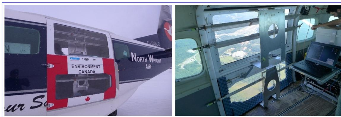
**Figure 1.** UMass Ku-band radar mounted in a modified Cessna 208 baggage door (Left). A single transmit antenna is mounted in the lower half and two receive antennas in the upper half (Right). Electronics for the system are mounted as a single rack easily transported between a variety of aircraft platforms.
