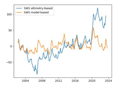
Thus, we computed groundwater storage variations for the present study based on our altimetry-based SWS results as GWS = TWS - RZSM - SWS(altimetry). Snow and ice can be neglected in the study region.
