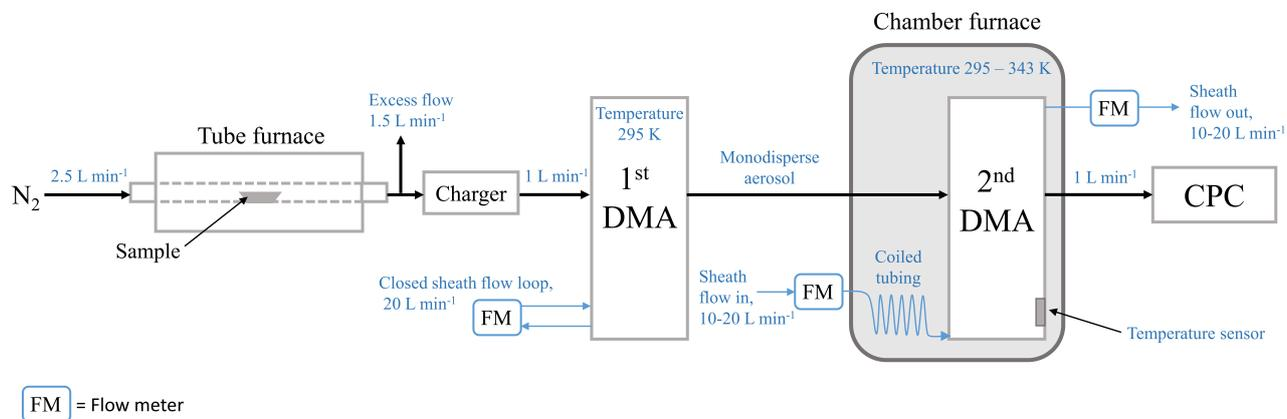
**Figure 1.** Schematic of the constructed tandem DMA setup.
