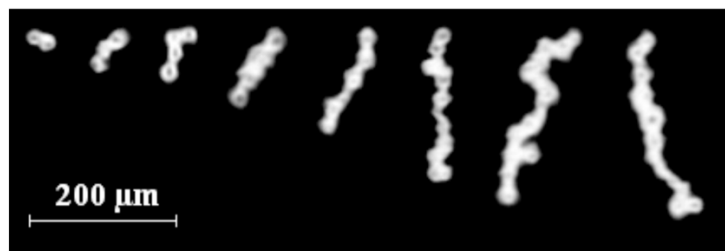
Fig. 10. Typical examples of chain-like aggregates ice crystals from 2 up to 15 individual frozen droplets.
