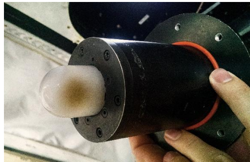
235 Figure S11. Strong aerosol contamination of the optic following the flight on 19 May, 2016.
