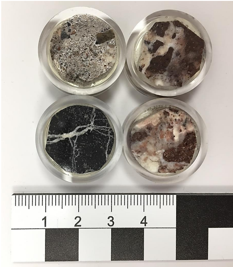
Figure S.10: Sample pucks of shattered clast samples (with salt filling) for SEM imagery. All samples are embedded in epoxy resin.
