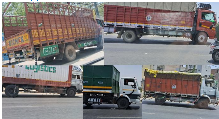
Figure S12: Random selection of photographs clicked while driving around Delhi. One can clearly see the white CNG cylinders mounted in the place where the fuel tank used to be during vehicle conversion. Photo credits: Kriti Annika Sinha
