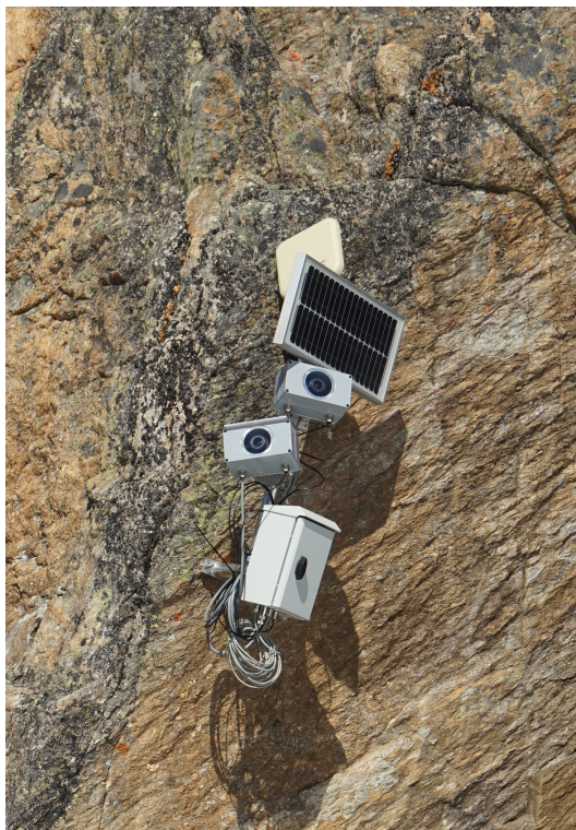
(a) Station with two cameras, bolted to a rock face at Lukschalp.
