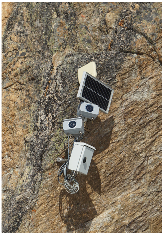
(a) Station with two cameras, bolted to a rock face at Lukschal. (b) Station with (initially) three cameras, mounted on a mast at Sattel.
