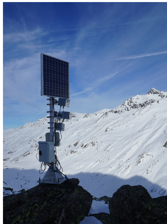
(a) Station with two cameras, bolted to a rock face at Lukschal. (b) Station with (initially) three cameras, mounted on a mast at Sattel.
