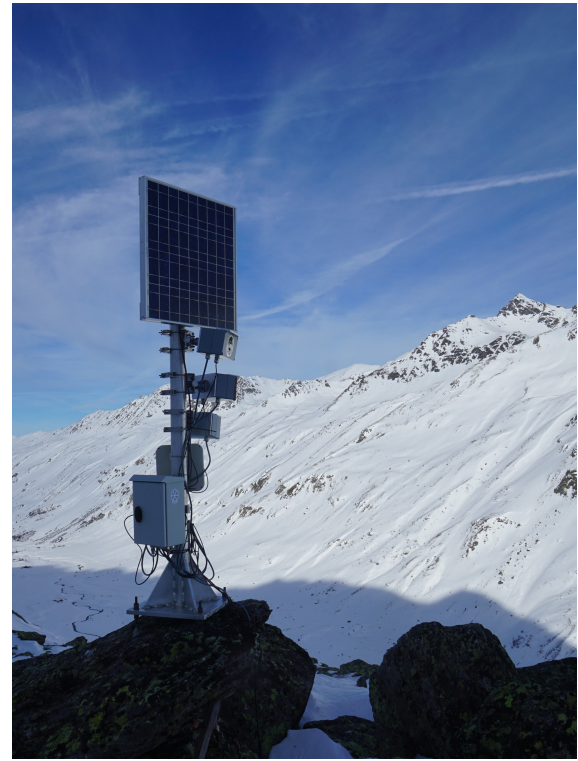
(b) Station with (initially) three cameras, mounted on a mast at Sattel.
