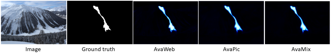
Figure 7. Example for an image from the SLF test that all three models solve solved well. The lighter the hue in the model predictions the higher the model certainty concerning the existence of an avalanche. In a close-up look the AvaWeb prediction exhibits more nuanced and detailed avalanche boundaries.
