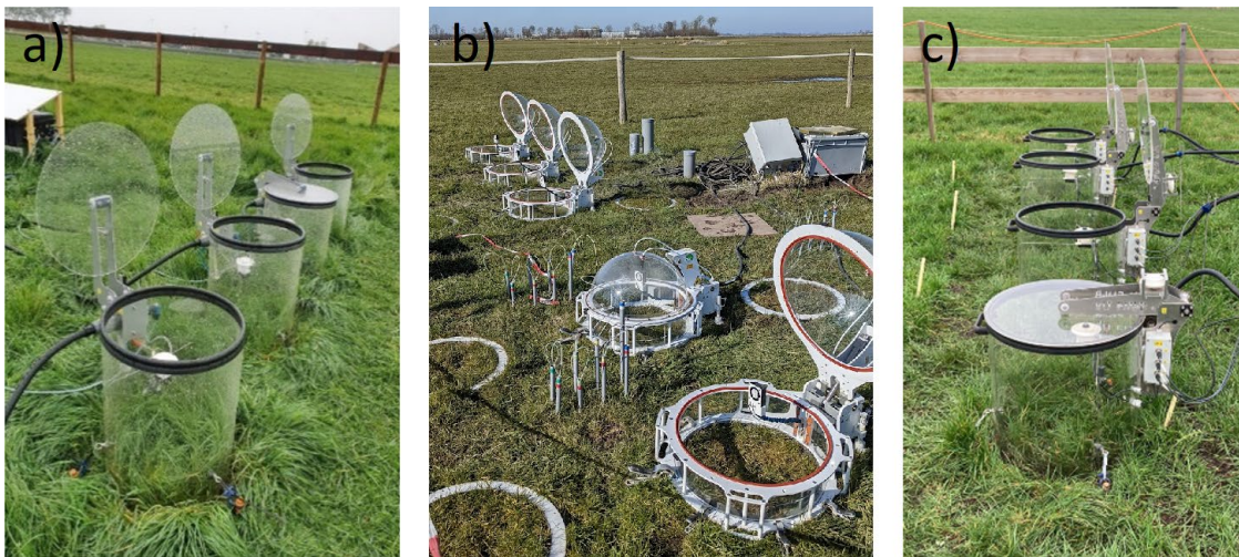
Figure 3. Transparent chamber systems: (a) VLUXpod, (b) Eosense eosAC-LT and (c) VLUXpod-L chambers
