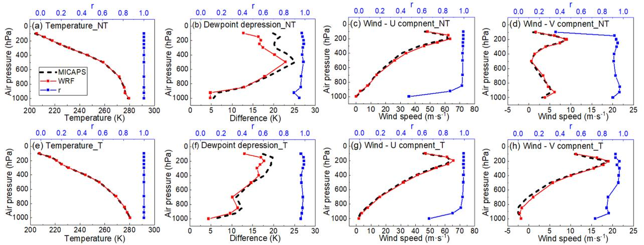
**Figure S1.** The vertical profiles of temperature (a and e), dewpoint depression (b and f), and the U (c and g) and V (d and h) wind components, averaged over the outer domain during NT (a-d) and T (e-h), are presented for both the WRF simulations (red lines for the Control experiment) and MICAPS (black lines), along with the spatial correlation between them at each vertical level (blue lines, upper axis).
