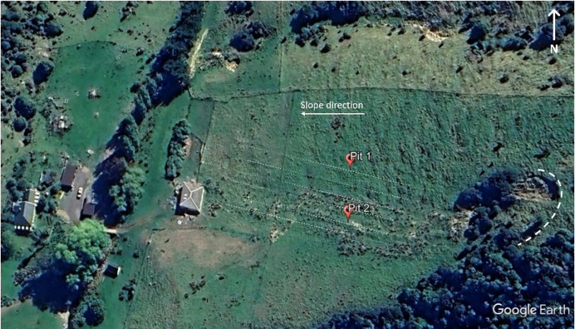
Figure 4: Location of soil pits. Raised mound positions are indicated by straight dashed lines. The origin of the landslide is indicated to the right of the image by the curved line. © Google Earth.
