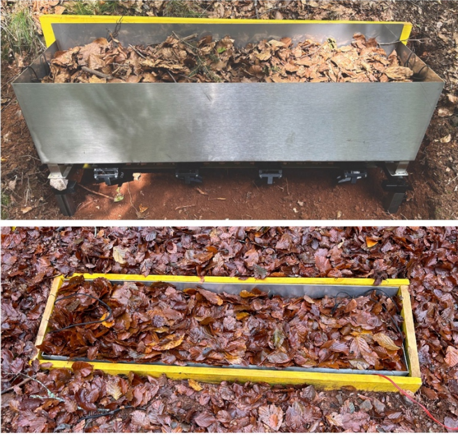
165 Figure 2: Top: Lysimeter container on the frame, bottom: fully installed FFGL aligned to the location.
