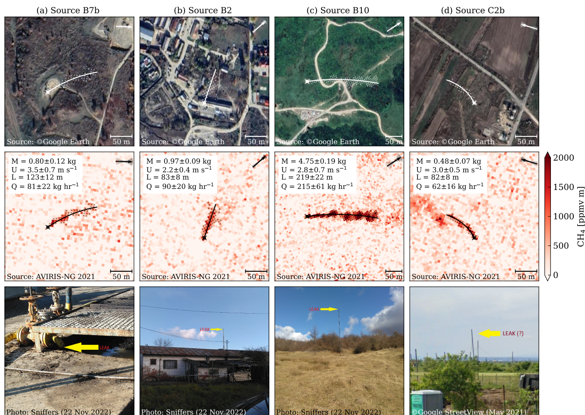
Figure 6. Four examples of \text{CH}_4 plumes at (a) an oil production site, (b) a processing facility and (c and d) from vent stacks in the open field observed in 2021. The panels from top to bottom show Google Earth imagery, AVIRIS-NG \text{CH}_4 maps with estimated emissions Q , and site photos with a yellow arrow indicating the emission point. M , U and L are integrated mass, wind speed and plume length. All uncertainties are 1\sigma . The maps show the detected plumes as dots and the plume center curve as line. The arrow in the top-right corner shows the wind direction from IFS analysis including the spread ( 2\sigma ) from the ERA-5 reanalysis as shaded area.
