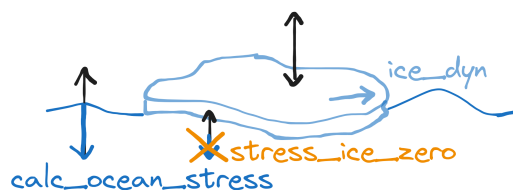
Figure 3. Stresses in between atmosphere, ocean, and sea ice and how the three switches described in Sec. 3.2.1 act on them.
