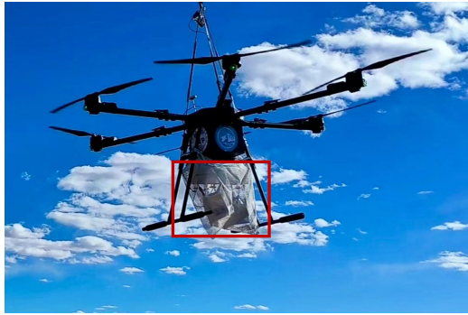
Figure 1. The design of the sampling system and its equipment on a UAV
