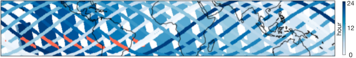
Figure 1. Illustration of the temporal and spatial match between Aqua–AIRS and TRMM–PR orbits. Orange represents the satellite trace segments, coincident within a time window of \pm 20 minutes, for one specific day. The narrow swaths represent TRMM–PR orbits, while the broader swaths represent Aqua–AIRS orbits. Shades of blue indicate variations in sampling time difference.
