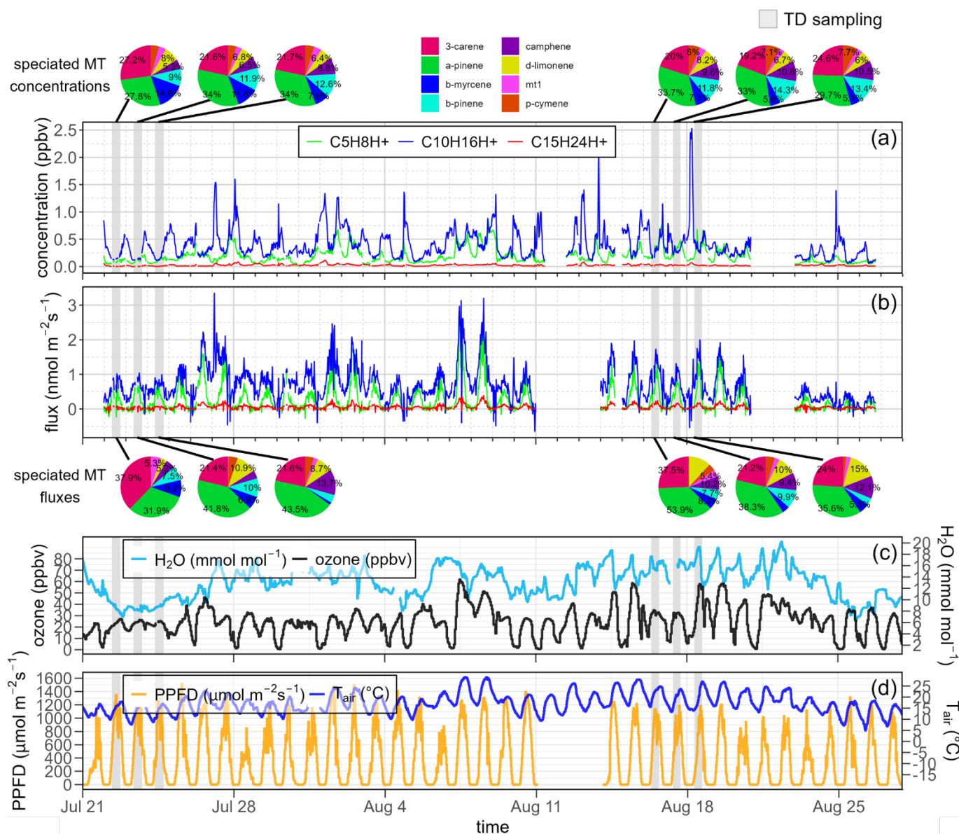
Figure 2: The 30-min BVOC concentrations (ppbv) and fluxes (nmol m -2 s -1 ) sampled at the 37 m BVOC inlet at ICOS Norunda, as well as related meteorological measurements. Shaded areas depict manual TD BVOC sampling periods at 37 and 60 m on the Norunda flux tower. The pie charts indicate the relative speciation of MT compound concentrations at 37 m (top) and fluxes (via SLG flux method) (bottom) as determined from the TD BVOC samples (percentages shown are >5%). (a) MT, isoprene, and SQT concentrations (ppbv) and (b) eddy-covariance derived fluxes (nmol m -2 s -1 ) from the Vocus PTR-ToF-MS. (c) Ozone concentration (ppbv) and water vapor (mmol mol -1 ). (d) PPFD (μmol m -2 s -1 ; at height 55 m) and air temperature (°C; at 37 m). Set of displayed measurements span from 21 July 2020 to 27 August 2020.
