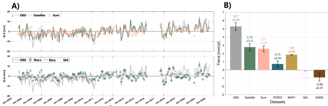
445 Figure 12. Monthly time series of sea level anomalies (left) and sea level rise rates (right; units: mm/yr). Each 446 color and type of line indicates the dataset (OBS: black solid line, Satellite: dark olive dotted line, Sum: salmon 447 pink circle, STERO: bluish green diamond, BARY: dark yellow dotted line, GIA: pale lavender dashed line, and 448 GNSS: dark brown).
