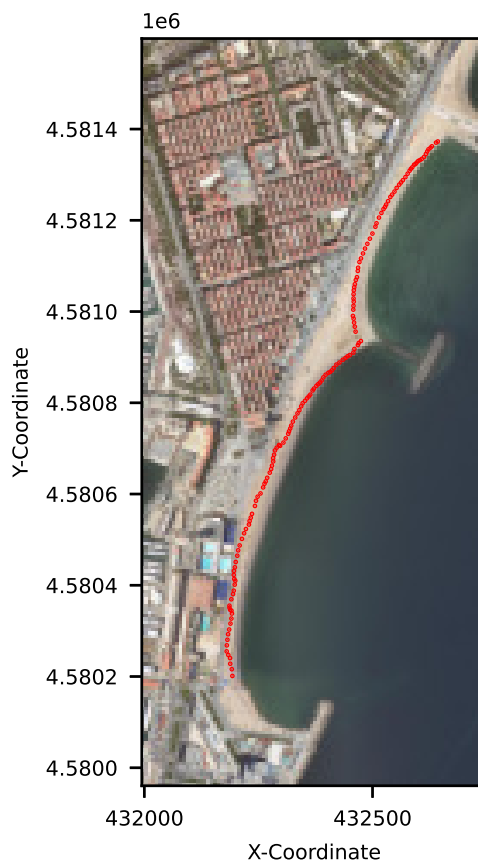
Figure 4. Example of figure received within the e-mail showing the magnitude of flooding, in this case for a high-intensity event. The red line shows the expected flooding line from the forecast. Orthophoto obtained from the ICGC WMS.
