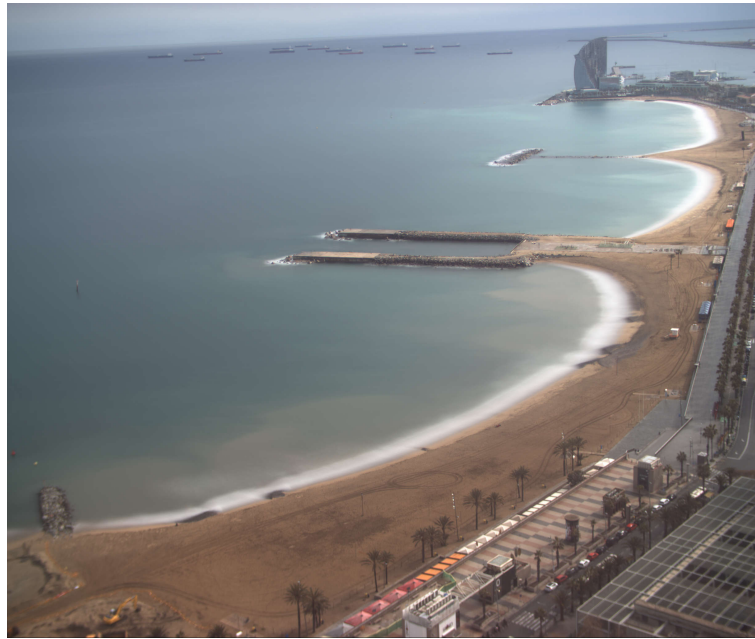
Figure 7. Time averaged ( timex ) image corresponding to April 3th, 2022. From top to bottom: SMSS and Barceloneta, which is the study area of the work, and Somorrostro beaches.
