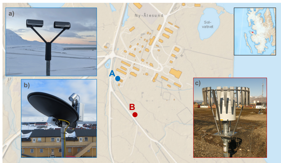
Figure 1. a) Parsivel, b) MRR, and c) Pluvio of the University of Cologne at Ny-Ålesund. The Parsivel and MRR are located on the roof platform of the AWIPEV atmospheric observatory (Fig. 1, location A) while Pluvio is installed in the field about 180 m away (Fig. 1, location B). The map of Ny-Ålesund and the map inlet showing the location of Ny-Ålesund in northwestern Svalbard are taken from https://toposvalbard.npolar.no by courtesy of the Norwegian Polar Institute.
