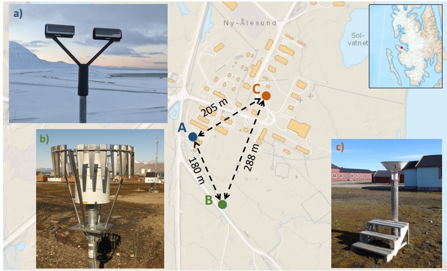
Figure 1. a) Parsivel and b) Pluvio of the University of Cologne at Ny-Ålesund. The Parsivel is located on the roof platform of the AWIPEV atmospheric observatory (location A), while Pluvio is installed in the field about 180 m away (location B). In addition, the MET Norway precipitation gauge (c) located in the center of Ny-Ålesund (location C) is shown. The map of Ny-Ålesund and the map inlet showing the location of Ny-Ålesund in northwestern Svalbard are taken from https://toposvalbard.npolar.no by courtesy of the Norwegian Polar Institute.
