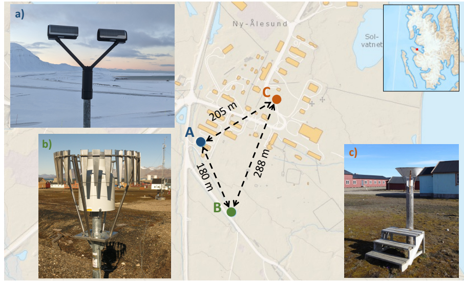
Figure 1. a) Parsivel and b) MRR, and c) Pluvio of the University of Cologne at Ny-Ålesund. The Parsivel and MRR are is located on the roof platform of the AWIPEV atmospheric observatory (Fig. 1, location A), while Pluvio is installed in the field about 180 m away (Fig. location B). In addition, the MET Norway precipitation gauge (c) located in the center of Ny-Ålesund (location BC) is shown. The map of Ny-Ålesund and the map inlet showing the location of Ny-Ålesund in northwestern Svalbard are taken from https://toposvalbard.npolar.no by courtesy of the Norwegian Polar Institute.
