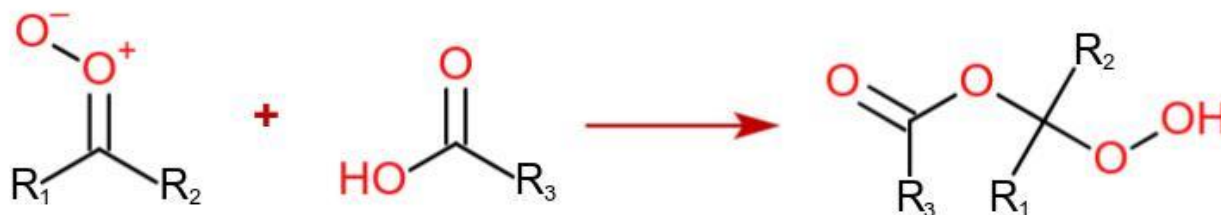
Scheme 1. The Criegee Intermediate + Carboxylic Acid reaction forms an \alpha -acyloxy hydroperoxide accretion product.
